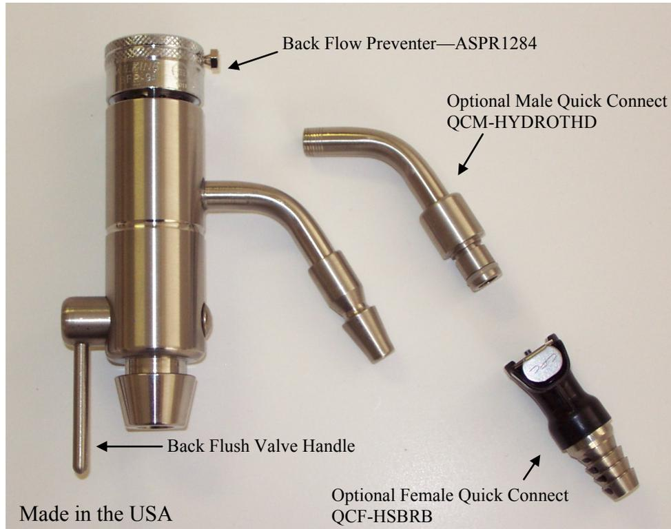
**INSTALLATION:** To install simply attach to any sink faucet with garden hose type threads. Attach suction hose to 90 degree elbow on side of unit. Next attach a splash tube to outlet at the base of the Hydro Aspirator.
